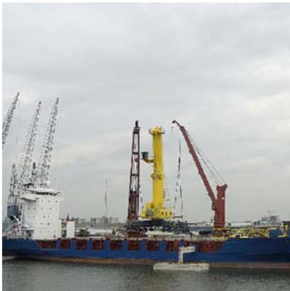
The ship used will be the MV Palessa or one of its sister ships designed to transport heavy cargo. These ships, built around the year 2000, are 118 metres long and can transport up to 7,000 tonnes of cargo.
